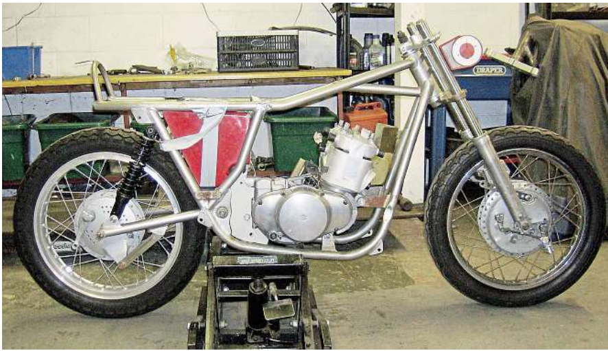
Checking fork rake and we found a lazy 29° – we want 27.
