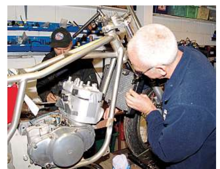
Checking for Rickuki radiator fit.
