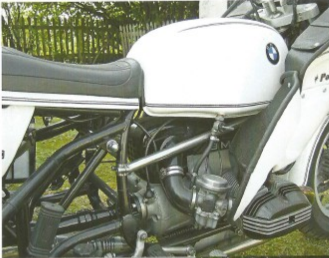
Close-up view of the frame strengthening.
