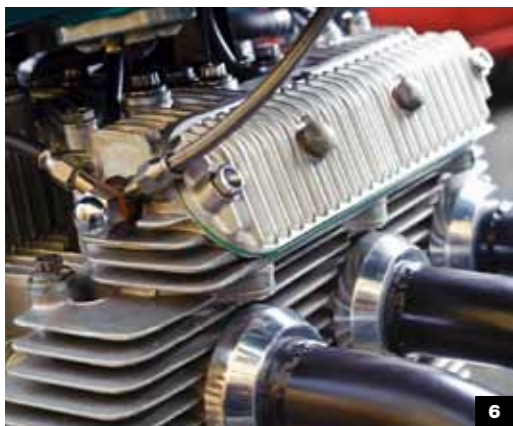
1 Plaque marks site of former tacho drive 2 Original side-entry plug no longer required 3 Widened Hinckley T-bird guard 4 Under-seat treats: Malarkey oil tank, mini battery with charge point, minimal wiring 5 ISR six-piston caliper gives power and feel. Lockwiring keeps it that way 6 Pressure-side oil feed to valvegear, milled-from-solid inspection cover, neat and tidy exhaust headers 7 Kickstart is a fusion of T150 and CB750. The 'Malarkey pin' on the right locks the whole shebang in the kicking position using a hidden spring 8 Polished and lightened tappets, with the golden glimmer of titanium collars 9 Flimsy 1969 number stays snug in recessed plate 10 Aftermarket holder, original lens. Mudguard is nine inches shorter than stock 11 Alternator wiring nips quietly across the gap into the frame tube 12 Rearset fofoests are pretty far back
