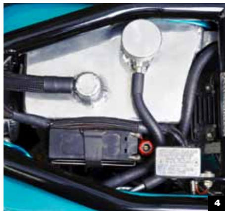
1 Plaque marks site of former tacho drive 2 Original side-entry plug no longer required 3 Widened Hinckley T-bird guard 4 Under-seat treats: Malarkey oil tank, mini battery with charge point, minimal wiring 5 ISR six-piston caliper gives power and feel. Lockwiring keeps it that way 6 Pressure-side oil feed to valvegear, milled-from-solid inspection cover, neat and tidy exhaust headers 7 Kickstart is a fusion of T150 and CB750. The 'Malarkey pin' on the right locks the whole shebang in the kicking position using a hidden spring 8 Polished and lightened tappets, with the golden glimmer of titanium collars 9 Flimsy 1969 number stays snug in recessed plate 10 Aftermarket holder, original lens. Mudguard is nine inches shorter than stock 11 Alternator wiring nips quietly across the gap into the frame tube 12 Rearset fofoests are pretty far back
