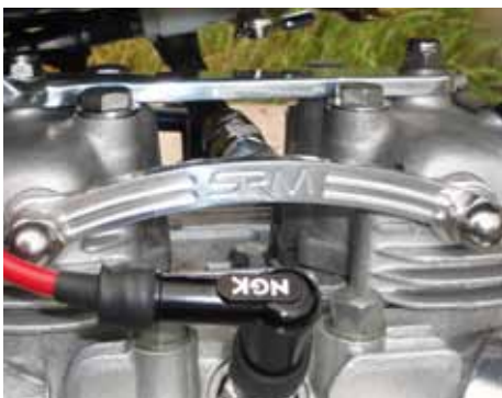
The carb / frame tube interception has been neatly handled, and the rocker oil feed is a beauty, too!
