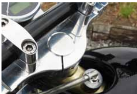
The oil goes in here. Unusually, the engine's oil inhabits all of the frame tubes, not just a central spine. Harder to fabricate, obviously, but saves significantly on weight and bulk
