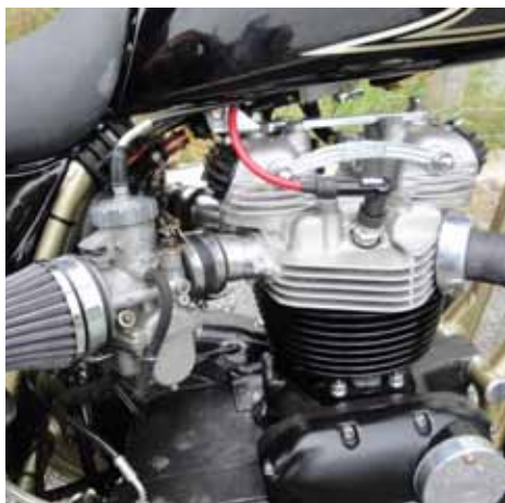
The carb / frame tube interception has been neatly handled, and the rocker oil feed is a beauty, too!
