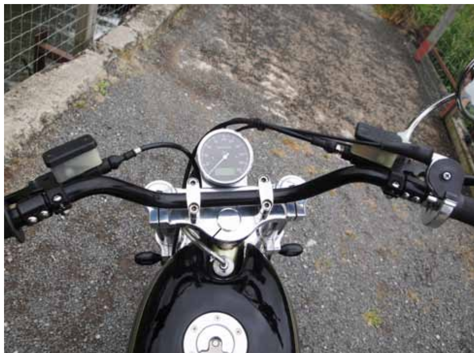
A view from the bar shows off the singular instrument and the equally singular controls. Hydraulic clutch and the neatest switchgear you'll see this year
