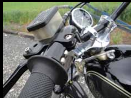
Duplicate hydraulics and controls. Superb light throttle and clutch, and a most effective anchor also
