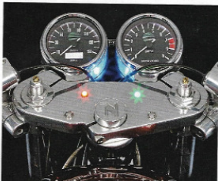
ABOVE: Peashooter 'silencers' are misnamed; quieter ones are planned. Corbin seat is a Commando aftermarket part. BELOW: Clocks are Smiths electronic items; milling the clamps off the Buel top yoke left handy holes for charge/neutral lights and clock menu switches. MkIII B50 gearbox, built brand new, with Quaife five-speed internals, has the gearchange was on the 'modern' side in keeping with the ethos of the bike
