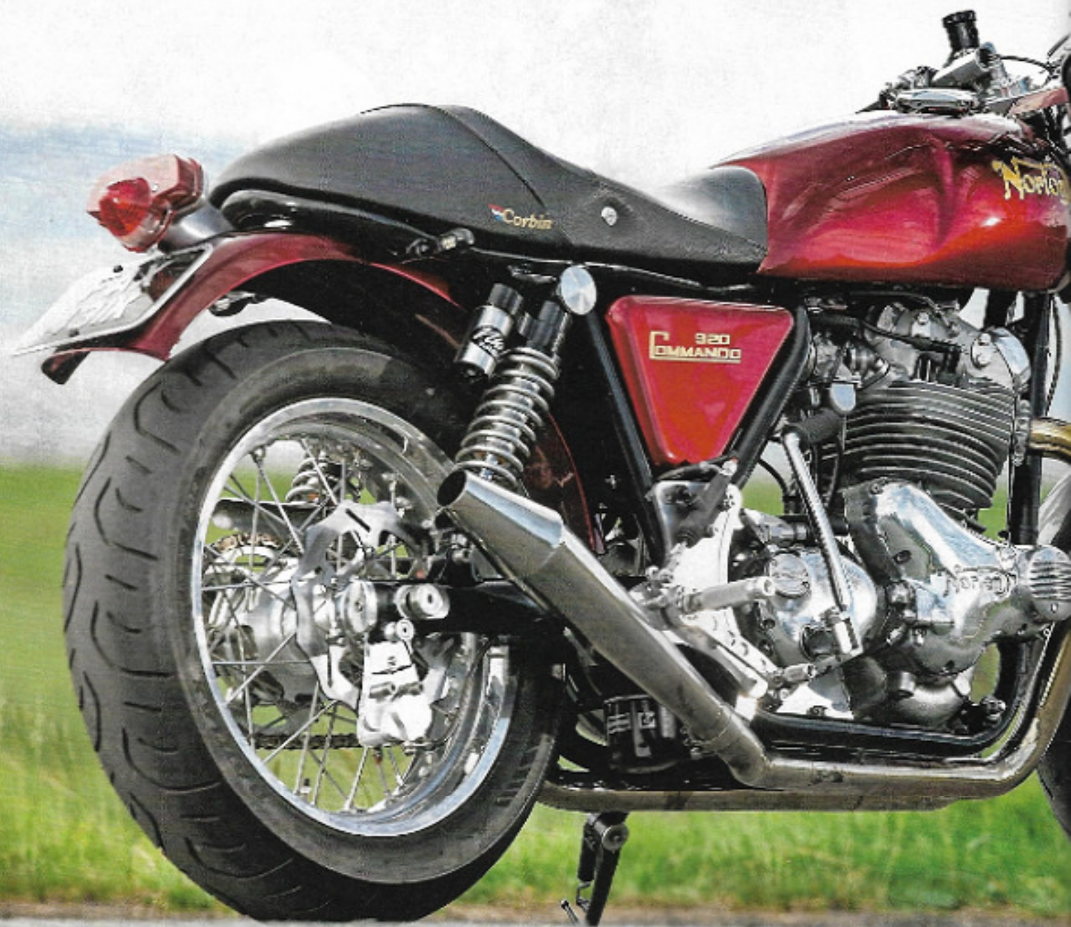
ABOVE: Peashooter 'silencers' are misnamed; quieter ones are planned. Corbin seat is a Commando aftermarket part. BELOW: Clocks are Smiths electronic items; milling the clamps off the Buel top yoke left handy holes for charge/neutral lights and clock menu switches. MkIII B50 gearbox, built brand new, with Quaife five-speed internals, has the gearchange was on the 'modern' side in keeping with the ethos of the bike
