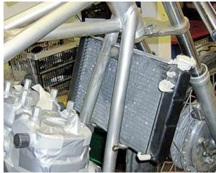
Radiator mounted at last!
